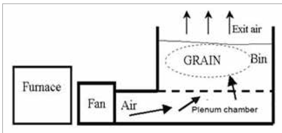
**Figure 3. Typical schematic design of flatbed dryer**
