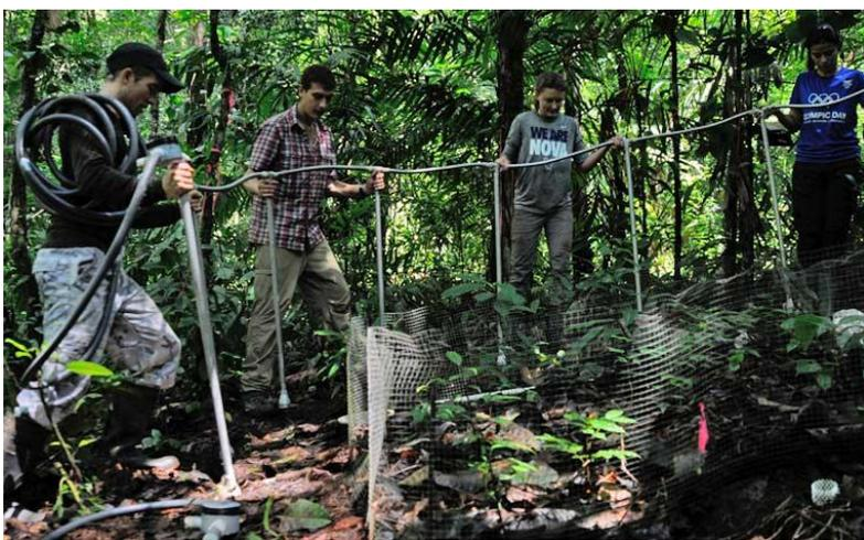
Researchers set up equipment in Panama to measure the release of soil carbon. Soils were artificially heated to imitate future global warming in the tropics. Image by Geetha Iyer.
